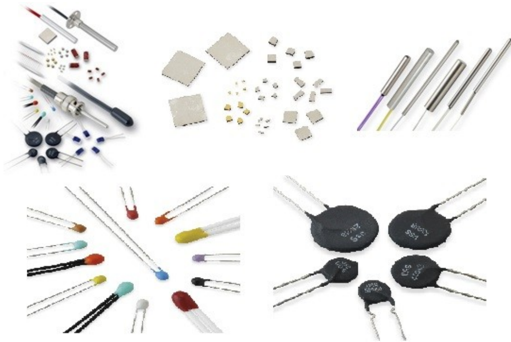
Fig. 1. Different types of thermistors
